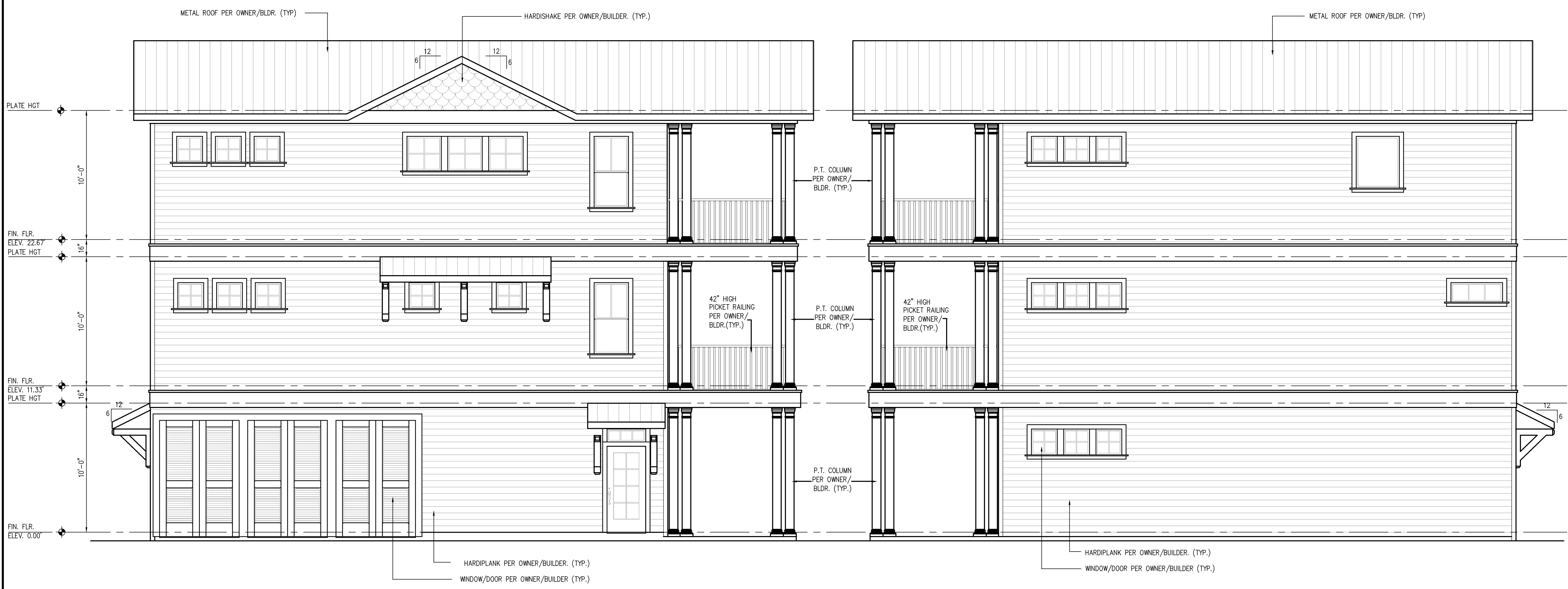
RIGHT SIDE ELEVATION SCALE: 1/4"=1'-0"
